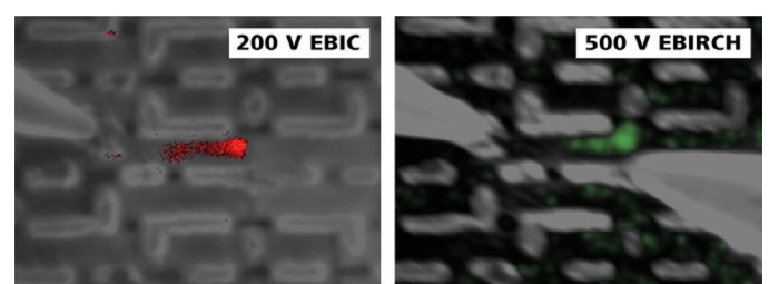
Figure 15 Comparison of EBIRCH, EBIC, and overlay of the two data sets. In the left image, EBIRCH data are overlaid with green; in the right EBIC is overlaid in red.
