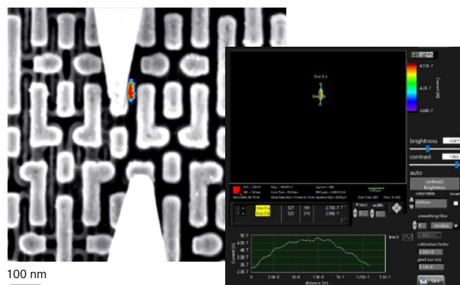
Figure 2 EBIRCH result for SRAM cell taken to 3 V of stress between source and gate, without compliance. Left image is SEM + EBIRCH overlay; right is quantitative analysis. This analysis showed a doubling of the current across the device, from 280 nA to 480 nA, due to beam stimulation.
