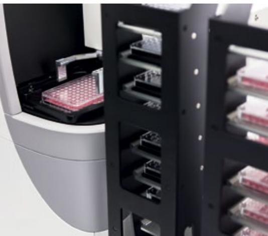
**Fig. 1:** Proper integration of robotic loaders into imaging systems can boost the degree of automation and thereby throughput. However, this is only one automation aspect and robotics must work seamlessly together with all other components of the system.
