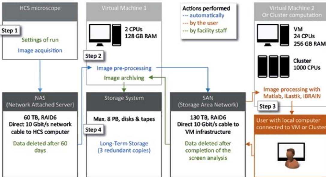
Fig. 2: Workflow for High-Content-Screening.
