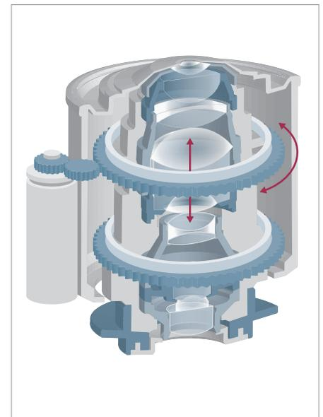
**Figure 2** Autocorrection objectives. ZEISS Celldiscoverer 7 objectives include an autocorrection ring to automatically adapt to bottom material and thickness. This way an optimal image quality is ensured for all sample carriers in every acquisition.
