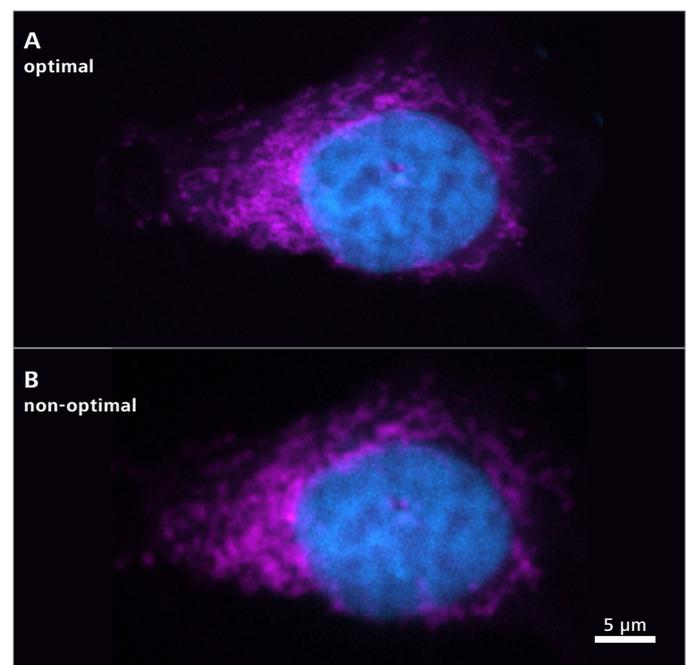
**Figure 4** Comparison of image quality and different laser powers under A: optimal autocorrection ring settings (1,020 μm). Laser power: DAPI (blue) 2.5% 405 nm, Mitotracker (magenta) 1.5% 561 nm; B: non-optimal autocorrection ring settings (210 μm). Laser power: DAPI (blue) 25% 405 nm, MitoTracker™ Red (magenta) 80% 561 nm.
