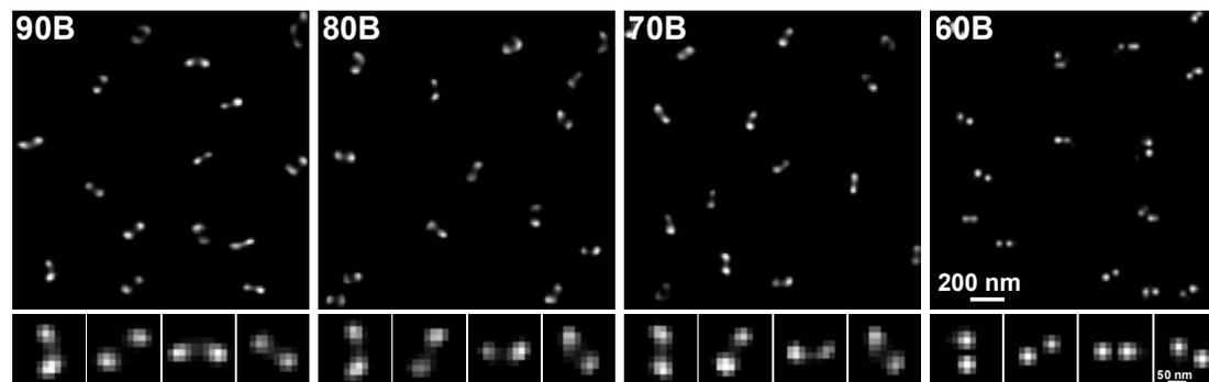
GATTA-STED Nanoruler 90B, 80B, 70B and 60B (GATTAquant, Germany) were imaged and processed with Elyra 7 Lattice SIM<sup>2</sup> mode with a 63x/1.4 oil objective. Distances of 90 nm, 80 nm, 70 nm and 60 nm are resolved.
